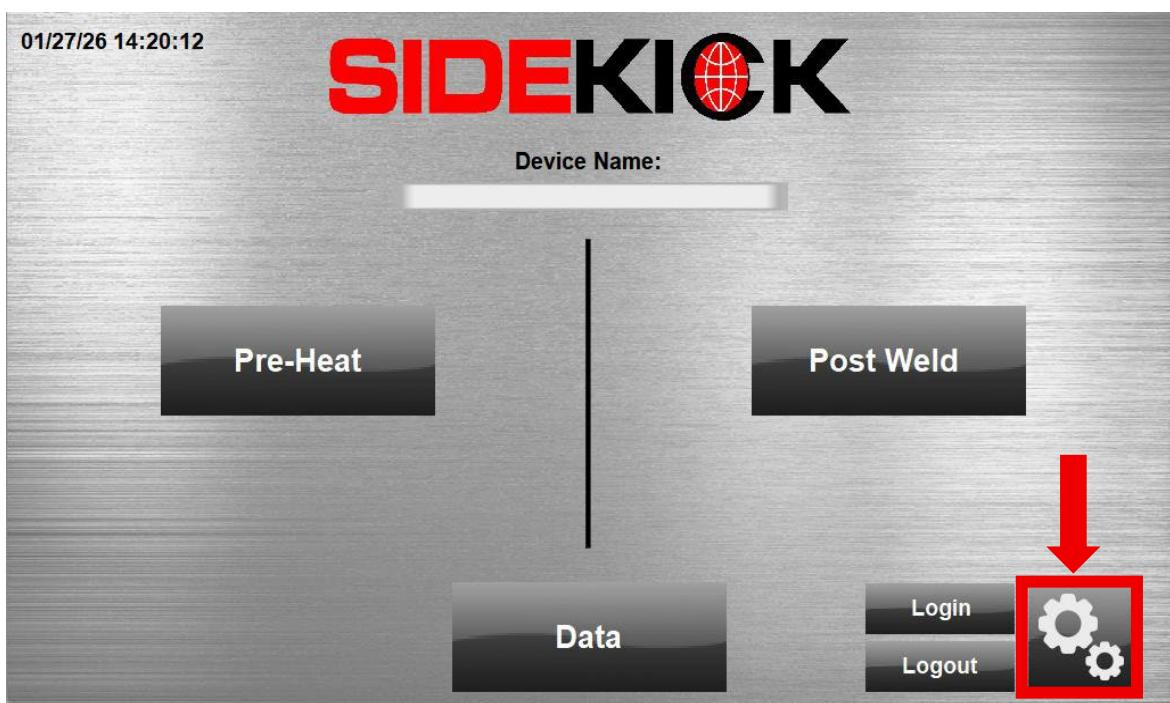
3. Select the “Calibration” button at the bottom of the screen.
