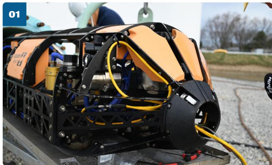
operational, autonomously navigating tanks containing gasoline, diesel, jet fuel, renewables, and other products. The data collected during these sessions is immense – phased-array ultrasonic data, tank-bottom elevation and settlement mapping, and internal visuals. This approach allows terminal operators to maintain operations, stay aligned with API 653 and EEMUA 159 requirements, reduce downtime, eliminate confined space entry, and avoid emissions associated with draining and cleaning.
