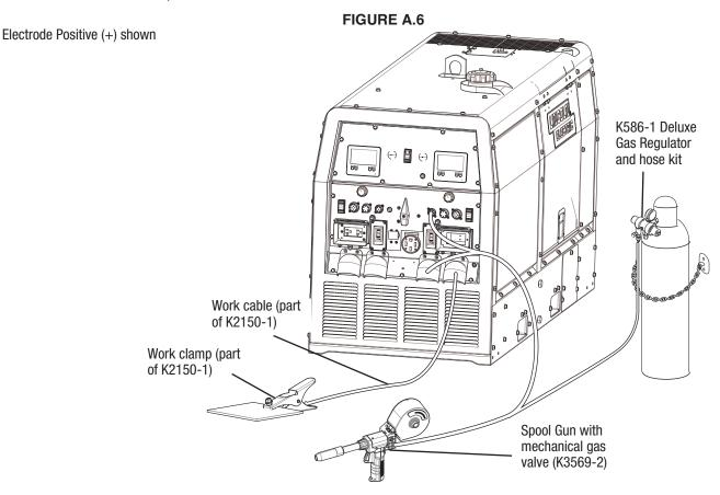
In the spool gun mode, the weld output is controlled by the trigger of the spool gun. The knob on the Dual Maverick display sets voltage and the spool gun knob sets wire feed speed. Rotating the knob on the spool gun adjusts the work point (wire feed speed). Spool gun modes have the option of being "synergic" (when the wire feed speed is changed, the voltage is automatically modified up or down to maintain a similar arc length).
