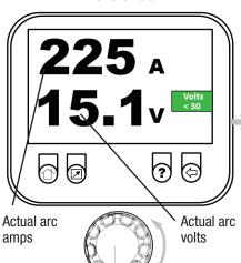
Stick Welding Basic 5 seconds after arc goes out
