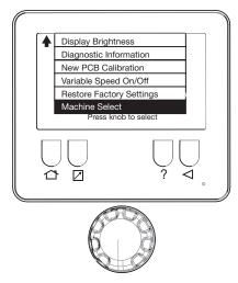
Enter the correct K# and Code # for the welder the PCB is being installed on. K# and Code # can be found above the top name plate("Machine Information Above"). Failure to enter the correct K# and Code # may result in permanent damage to the welder.
