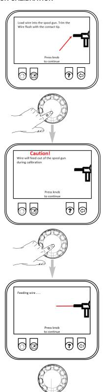
This screen will remain for approximately 5 seconds as the wire feeds. During this process, the wire coming out of the spool gun will grow longer as a visual representative.
