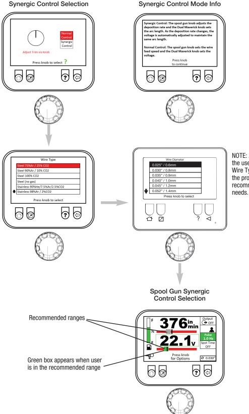
NOTE: After selecting Synergic Control, the user is required to select their desired Wire Type and Wire Diameter. This allows the program to calculate the recommended range for their welding
