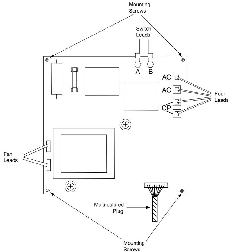
11. Using a 7mm Nut driver, remove the four mounting nuts from the corners of the Input Board. Be careful not to lose the washer behind each nut. Input Board can be removed after these four nuts are removed.
