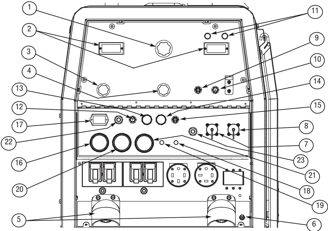
**1. OUTPUT CONTROL-** The OUTPUT dial is used to preset the output voltage or current as displayed on the digital meters for the five welding modes. When in the Arc Gouging or CV-WIRE modes and when a remote control is connected to the 3-Pin or 14-Pin Connector, the auto-sensing circuit automatically switches the OUTPUT CONTROL from control at the welder to the remote control.
