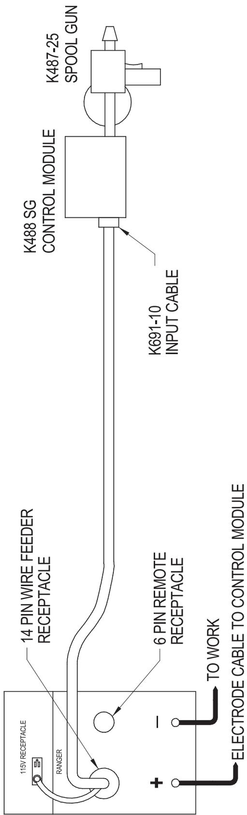
**CAUTION:** BE SURE THAT CONTROL MODULE MODE SWITCH IS IN THE "LINCOLN" (CONTACT CLOSURE) POSITION BEFORE ATTEMPTING TO OPERATE CONTROL MODULE. INCORRECT SWITCH POSITION COULD RESULT IN DAMAGE TO THE CONTROL MODULE AND/OR POWER SOURCE.
