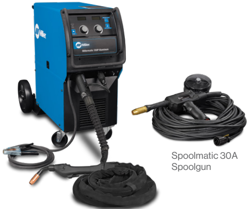
Millermatic 350P Aluminum, XR-Aluma-Pro Push-Pull Gun
