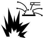
**WELDING SPARKS can cause fire or explosion.**
