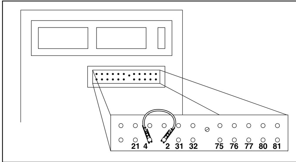
**FIGURE F.8 - Jumper Wire Connection Points**
