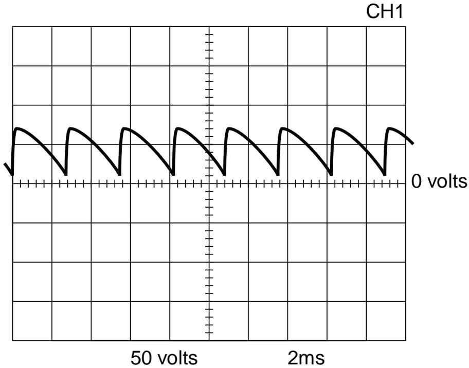
This is the typical DC open circuit voltage waveform generated from a properly operating machine. Note that each vertical division represents 50 volts and that each horizontal division represents 2 milliseconds in time.
