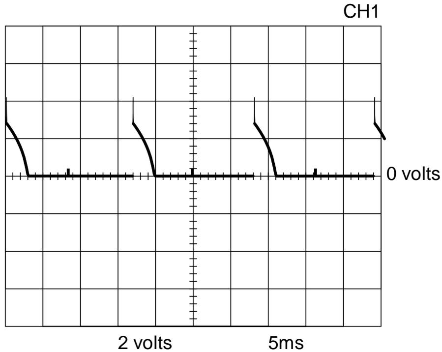
This is the typical SCR gate pulse voltage waveform. The machine was in an open circuit condition (no load) and operating properly. Note that each vertical division represents 2 volts and that each horizontal division represents 5 milliseconds in time.
