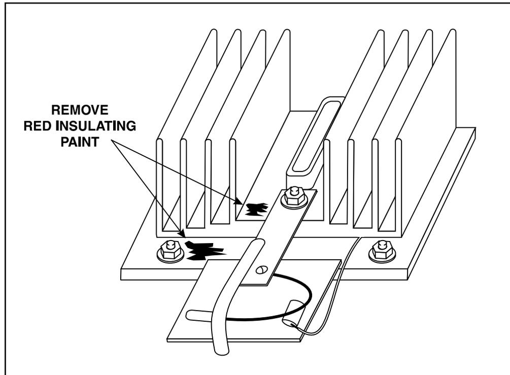
**FIGURE F.13 - Heat Sink Test Points.**
