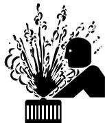
7.h. To avoid scalding, do not remove the radiator pressure cap when the engine is hot.
