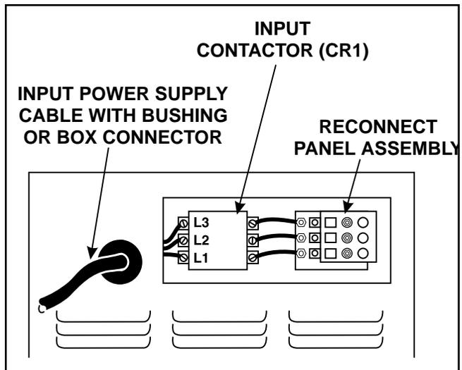
**FIGURE A.3 - Input Power Supply Connections**
