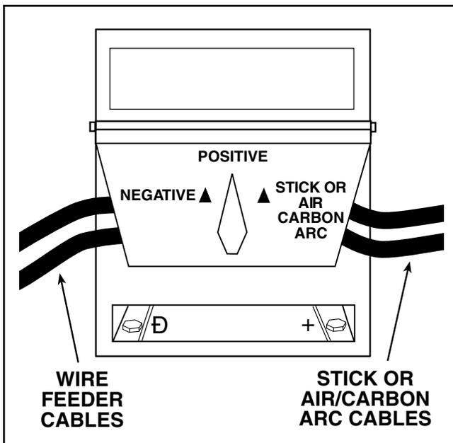
FIGURE C.1 - MULTI-PROCESS SWITCH
