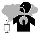
7.b. Operate engines in open, well-ventilated areas or vent the engine exhaust fumes outdoors.
