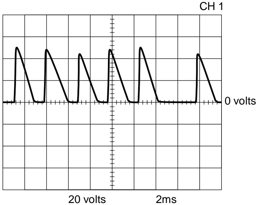
This is NOT the typical DC output voltage waveform. One output SCR is not functioning. Note the “gap” in the waveform. One SCR gate is disconnected to simulate an open or non-functioning output SCR. Each vertical division represents 20 volts and each horizontal division represents 2 milliseconds in time.
