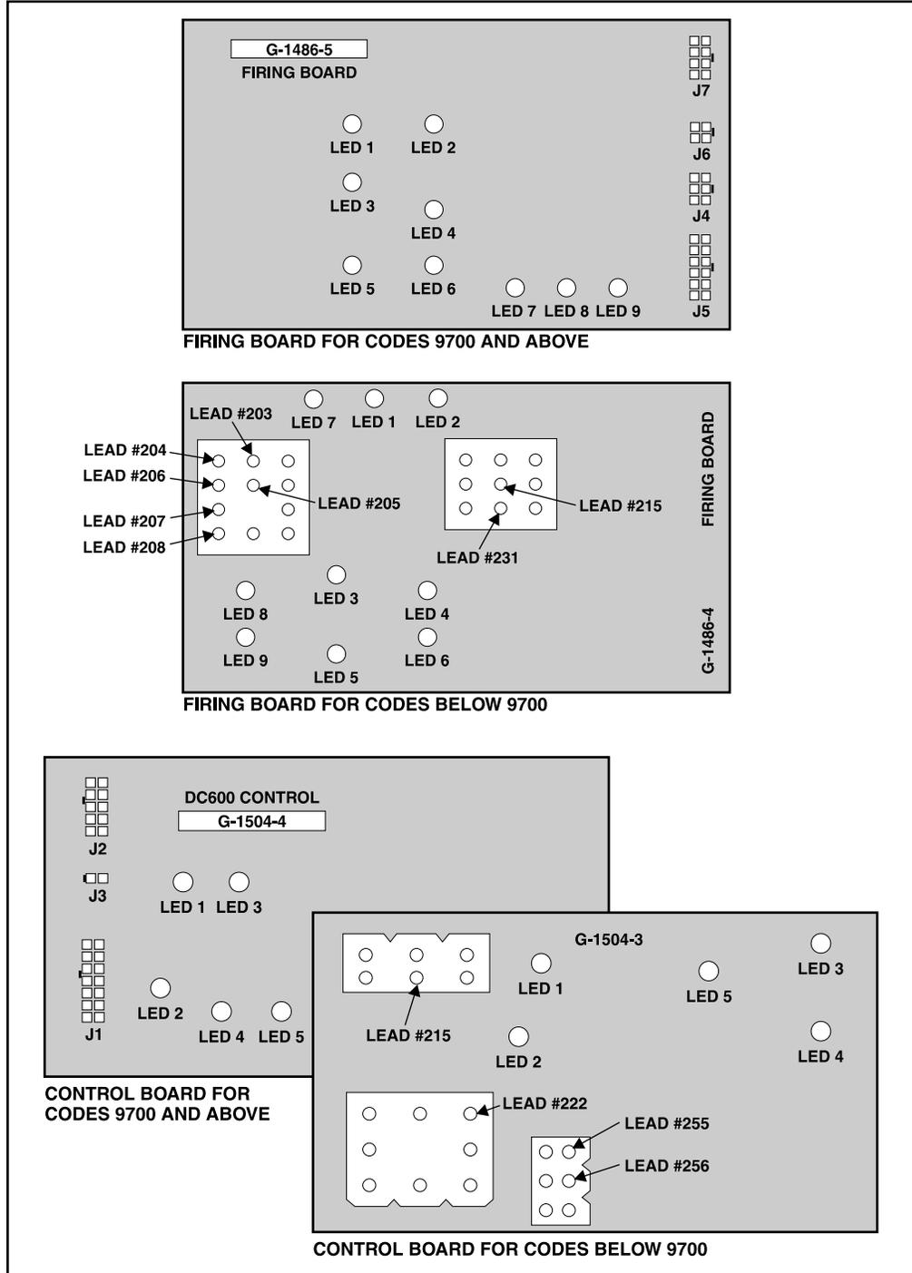
FIGURE F.12 - Firing Board and Control Board Molex Plug Locations.
