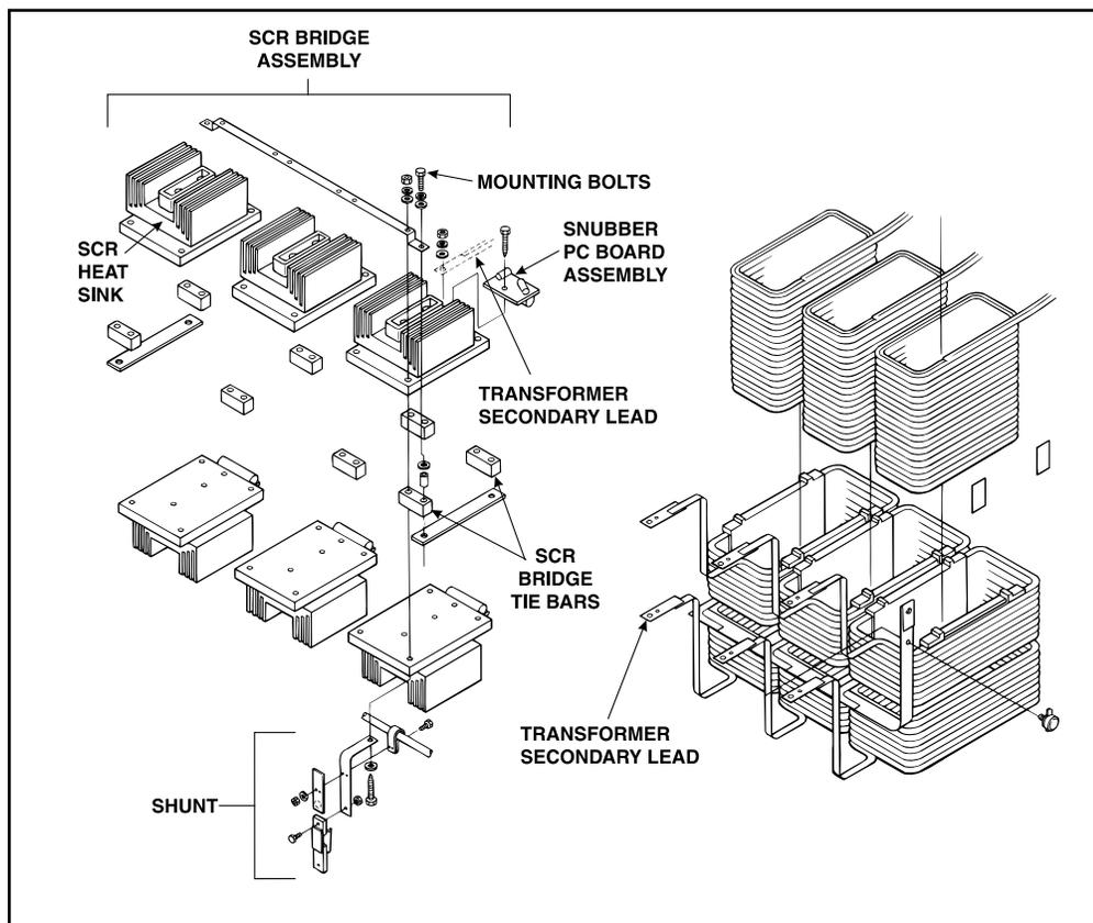
**FIGURE F.19 - Individual Heat Sink Removal**
