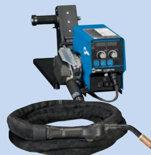
**Synergic pulsed MIG.** As you increase/decrease the wire feed speed, the pulse parameters increase/decrease, matching the right amount of power output to match the wire speed, eliminating the need to make additional adjustments.
