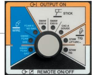
**LED process indicator.** Front panel process selections are illuminated with an LED that identifies the active process. This enables the selected weld process to be seen at a distance from the power source.
