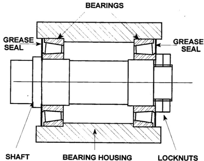
*Figure 6 Roller Bearing*
