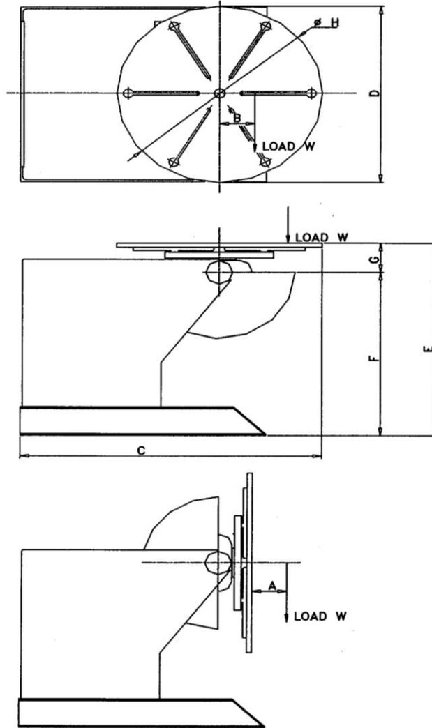
ROTATION TORQUE (R) IS A STRAIGHT FORWARD CALCULATION OF LOAD (W) X ECCENTRICITY (B) BUT TO ENSURE AN ACCURATE FIGURE FOR TILT TORQUE (T) IT IS IMPORTANT TO USE THE FULL DISTANCE TO THE PIVOT POINT. THIS IS OBTAINED BY ADDING TOGETHER THE CENTRE OF GRAVITY (A) AND TABLE PIVOT DISTANCE (G). THEREFORE :-
