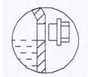
Screw out the plug screw at the point marked with this symbol.
