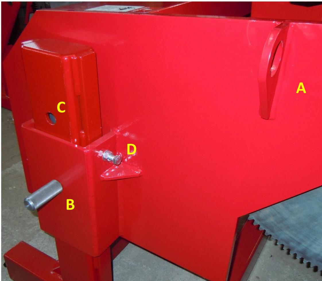
The table can then be raised or lowered by using the crane, so that hole C lines up with the lock pin (B) holes. Pin B on both sides of the machine can then be replaced. Once pins B are fully in place on both sides, then the weight of the table can be taken by the pins and the crane removed. Tighten the 4 bolts D (2 on either side of the machine), this will prevent any movement of the positioner inside the height adjustment sleeve.
