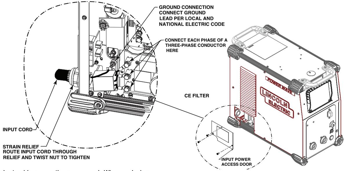
On some models, toroids are on the power cord. When replacing the power cord, it is important to put the toroids on the new power cord in the same location and with the same number of turns.
