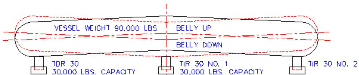
FIGURE 4 - INHERENT OVERLOAD: LONG VESSEL, BENT CENTERLINE, THREE ROLL UNITS
