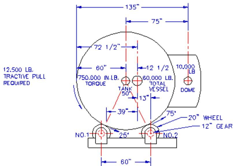
FIGURE 10 - VESSEL WITH ECCENTRIC CENTER-OF-GRAVITY
