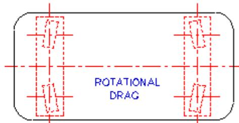
FIG. 3B - UNPARALLELED WHEELS DRAG
