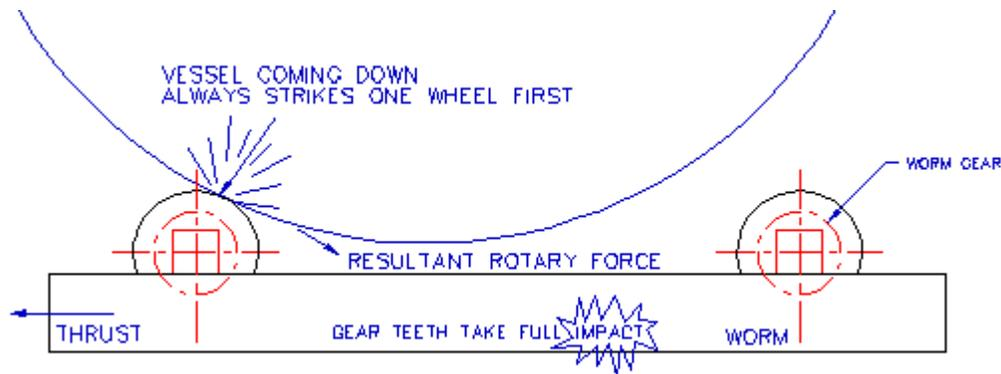
FIGURE 7 - WHEN LOADING THE VESSEL, IT ALWAYS STRIKES ONE WHEEL FIRST
