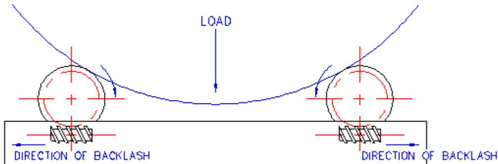
FIGURE 8 - BACKLASH ALWAYS LOADS OPPOSITELY AS THE VESSEL CRADLES INTO WHEELS
