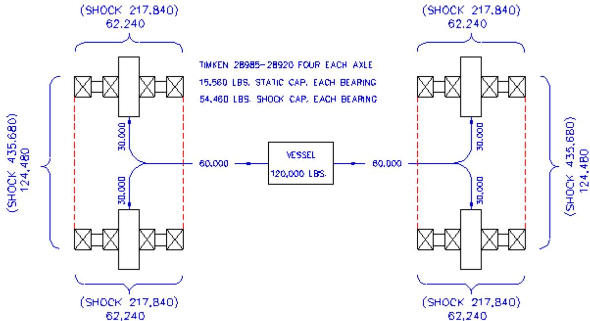
FIGURE 5 - LOAD DISTRIBUTION AND AXLE BEARING CAPACITY
