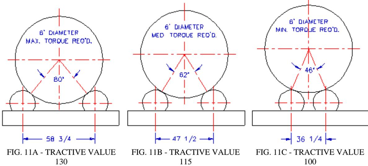
As shown in Figures 11A, B and C, a turning roll with adjustable center-distances will accommodate a given diameter vessel in more than one Center-Distance setting. For example, a PRESTON-EASTIN turning roll will cradle a 6-foot vessel in C-D settings of 36.25", 47.5" and 58.75". USE A SHORT CENTER DISTANCE WHENEVER POSSIBLE. Symmetrical, balanced vessels will safely cradle in contact angles between 45° and 60°.
