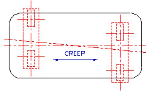
FIG. 2B - STAGGERED CHASSIS = ENDCREEP
