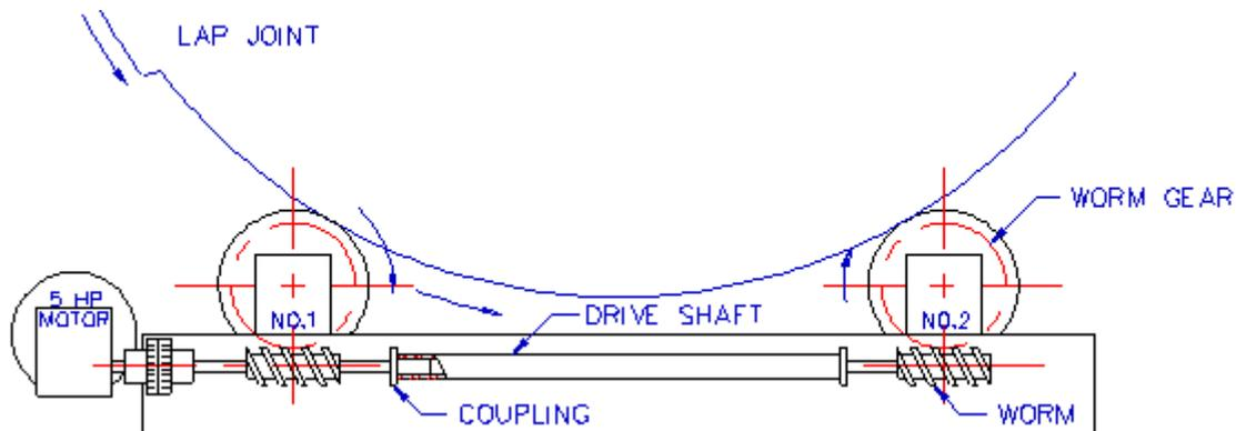
FIGURE 9 - NORMALLY, ONLY ONE WHEEL DRIVES WHEN ROTATING THE VESSEL
