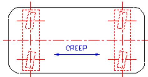
FIG. 2D - COCKED WHEELS IN CHASSIS = ENDCREEP
