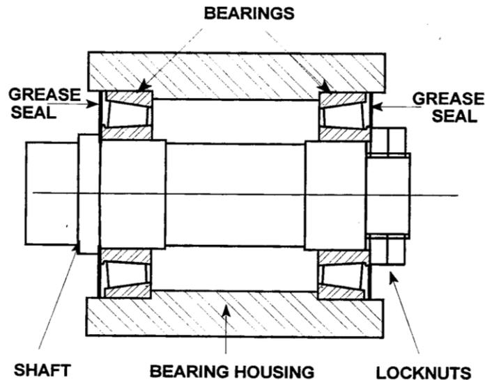
*Figure 6 Roller Bearing*
