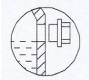
Screw out the plug screw at the point marked with this symbol.
