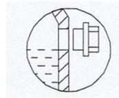
The oil level should be reduced to the level marked with this symbol (see D.1.1).
