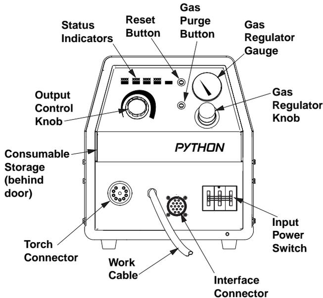
When preparing to cut or gouge, position the machine as close to the work as possible. Make sure you have all materials needed to complete the job and have taken all safety precautions. It is important to follow these operating steps each time you use the machine.
