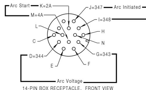
Users wishing to utilize the Machine Interface can order a K867 Universal Adapter (please adhere to the pin locations stated above) or manufacture a 14 pin MS connector cable assembly.
