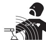
2.a. Electric current flowing through any conductor causes localized Electric and Magnetic Fields (EMF). Welding current creates EMF fields around welding cables and welding machines
