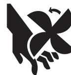
1.e. In some cases it may be necessary to remove safety guards to perform required maintenance. Remove guards only when necessary and replace them when the maintenance requiring their removal is complete. Always use the greatest care when working near moving parts.
