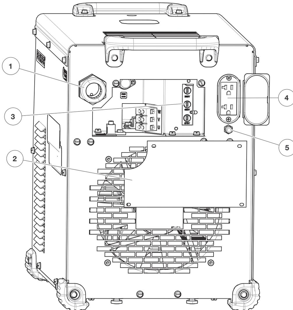
**INTERNAL CONTROLS - ENABLING VRD, MULTI-WELD AND CURRENT/VOLTAGE CALIBRATION**
