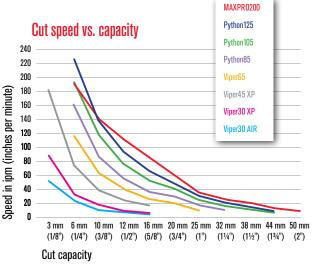
The recommended cut capacity is the thickness at which the system delivers good cut quality with torch travel speeds of about 500 mm (20") per minute. The severance cut capacity is the thickness at which the system can sever the metal but has poor cut quality with torch travel speeds approaching 125 mm (5") per minute.
