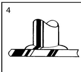
4 The weld gun is withdrawn from the weld stud leaving and the ferrule. The ferrule is broken away and discarded. Visually inspect weld.
