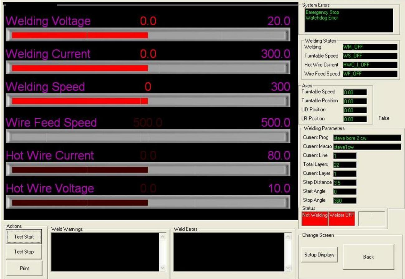
The majority of this screen is taken up with a live display of welding parameters, in the form of a bar chart. The actual values and required values are displayed. Alerts and alarms will warn of any parameter which fall out of the required range as set by the weld procedure. These are displayed at the bottom of the page.
