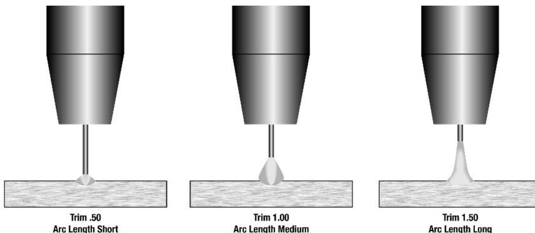
Most pulse welding programs are synergic. As the wire feed speed is adjusted, the Power Wave® S350 will automatically recalculate the waveform parameters to maintain similar arc properties.
