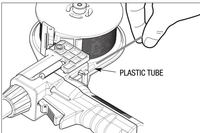
7. Push wire until end of wire exits back tube and enters front tube, passing between drive roll & pressure idler roll.
