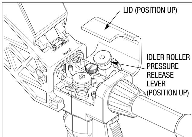
2. Take wrench (10mm) and loosen drive roll in a clock-wise direction while holding shaft with flat head screw driver. Flip drive roll and tighten in a counter-clockwise direction.
