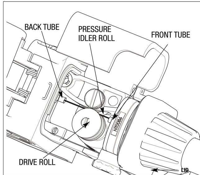
8. Push wire until wire end extends approximately 6" (150 mm) past end of gas diffuser. Re-engage idle roll pressure by pushing release lever down as shown above, then close lid.
