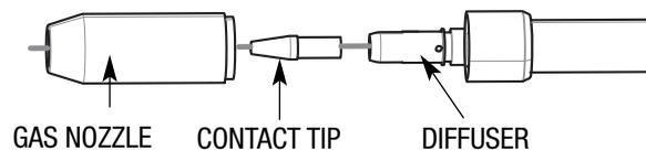
11. Cut off wire close to contact tip, then screw gas nozzle over the diffuser
