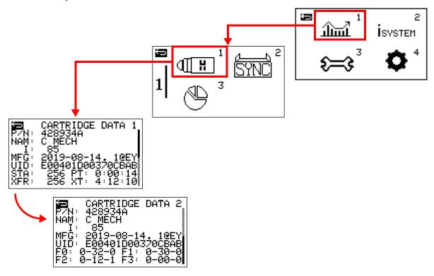
**P/N** – This field shows the part number (*nnnnnn*) and the version (X) of the Hypertherm cartridge.
