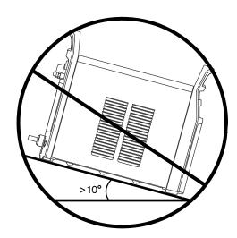
Do not put the plasma power supply on its side. Doing so can cause a blockage of the air circulation necessary to keep internal components cool.
