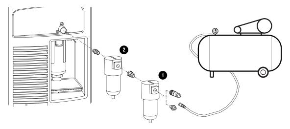
Figure 4 - Optional Hypertherm external filters
