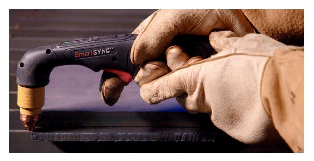
**2.** Pull the torch's trigger to start the arc. Stay at the edge until the arc has cut completely through the workpiece.
