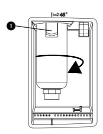
**6.** Gently turn and pull the filter element **2** out of the filter bowl. Be careful not to damage the O-ring **3** at the top of the bowl.
