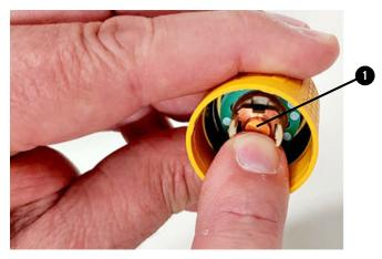
If the system shows an 0-32-0 or 0-32-1 fault code, install a new cartridge. Refer to When to replace the cartridge (fault code 0-32-n) on page 82.
