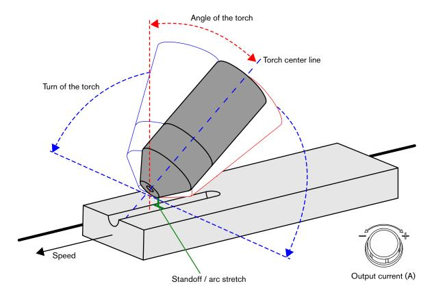
Figure 6 - Factors that change the gouge contour
