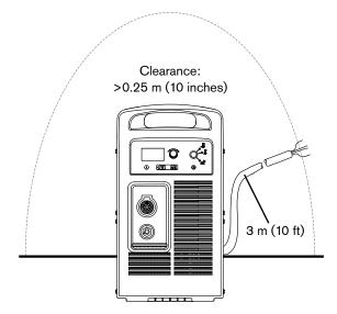
■ Put the plasma power supply on a stable, level surface before using. The plasma power supply can tip over if set at an angle greater than 10°.
