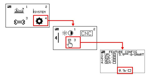
UPL – Set the low gas pressure detection feature to on or off. When you set this field to off, the system no longer shows the 0-20-0 fault code. For information on fault codes, refer to page 130. This field is on by default.
