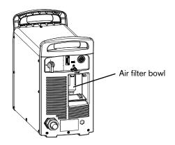
The built-in air filter must not take the place of sufficient external filtration. If you work in an environment that is extremely warm and humid, or if work site conditions introduce oil, vapors, or other contaminants into the gas line, install an external filtration system that cleans the gas supply before it gets into the plasma power supply.
