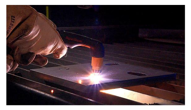
**5.** When the pierce is complete, drag the torch tip lightly across the workpiece to continue with the cut.
