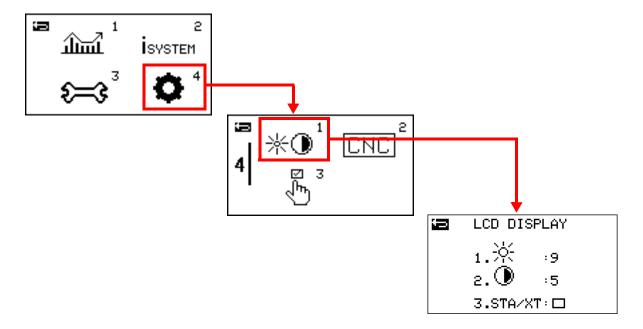
**4.** Turn the adjustment knob to adjust the value in the # field to increase or decrease the **brightness** of the LCD screen.
