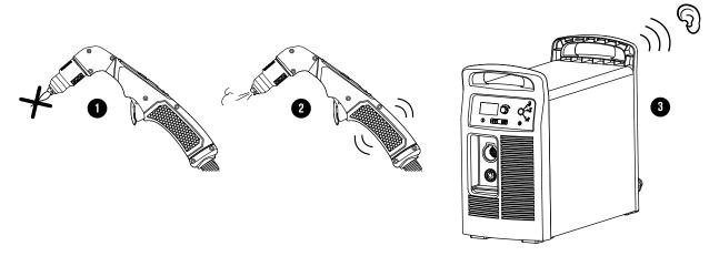
This feedback is a warning. It does not identify a fault condition. It tells you that the torch is unlocked and will fire a plasma arc the next time that you pull the trigger.
