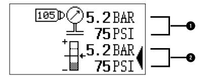
You can turn the adjustment knob to change the manual gas pressure setting during a gas test.
