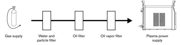
The filtering system must be installed between the gas supply and the plasma power supply.
