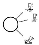
Operating mode button – The plasma power supply automatically sets the mode to Cut mode or Gouge mode related to the type of Hypertherm cartridge that you install. With a Hypertherm cutting cartridge installed, you can push this button to change from Cut mode to Expanded Metal mode. Refer to page 77 for more information.
