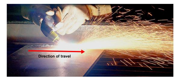
**6.** Change the position of the torch as necessary to get the gouge contour that you want. Refer to Change the gouge contour on page 114. Keep at least a small distance between the torch tip and the molten metal to increase cartridge life and prevent damage to the torch.
