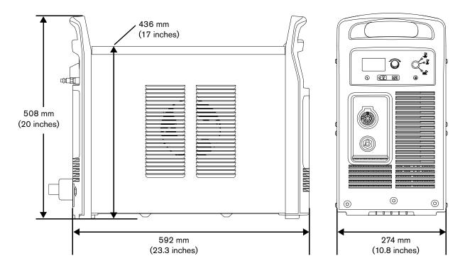
Figure 2 - Powermax105 SYNC dimensions
