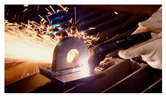
**9.** If it is necessary to adjust the flat side of the tip of the cartridge to complete the cut, lock the torch before you touch the cartridge.
