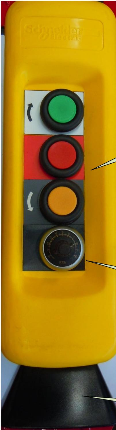
Rotation direction push buttons, forward reverse and stop.
