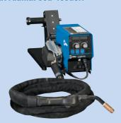
**Synergic pulsed MIG.** As you increase/ decrease the wire feed speed, the pulse parameters increase/decrease, matching the right amount of power output to match the wire speed, eliminating the need to make additional adjustments.
