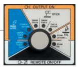
**LED process indicator.** Front panel process selections are illuminated with an LED that identifies the active process. This enables the selected weld process to be seen at a distance from the power source.
