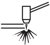
1. With the work clamp attached to the workpiece, hold the torch nozzle perpendicular (90°) to the edge of the workpiece. If you are using the shielded consumables, no standoff is needed. With unshielded consumables, maintain an approximate .08-inch (2 mm) standoff.
