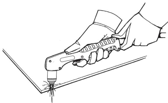
3. Drag the nozzle lightly across the workpiece to proceed with the cut. Maintain a steady, even pace.
