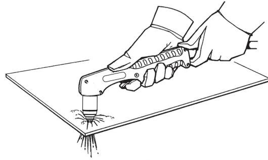
4. When the pierce is complete, drag the nozzle lightly along the workpiece to proceed with the cut.
