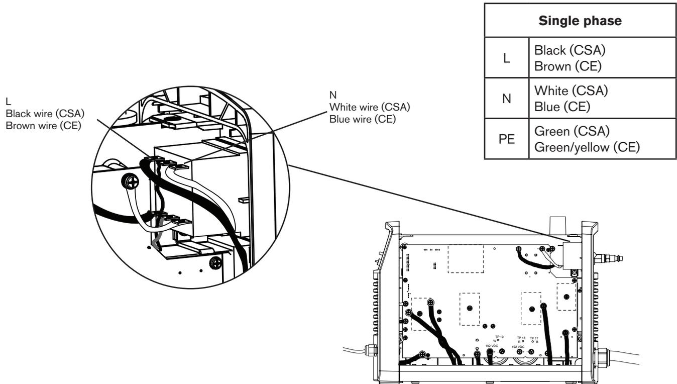
6. Remove the screw that holds the green wire to the heatsink.
