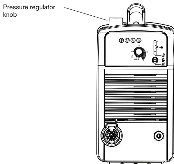
3. Turn the pressure regulator knob until the gas pressure LED shows a green bar in the center of the pressure bar.
