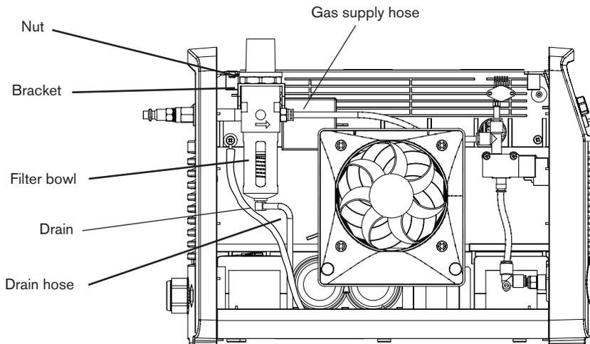
8. Remove the glass filter tube by twisting it and pulling gently until it releases.
