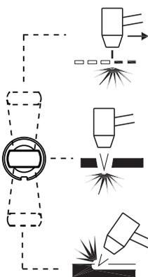
To cut expanded metal or grate (top position). Use this setting to cut metal with holes in it or for any job requiring a continuous pilot arc. Leaving the mode switch on this setting when cutting standard metal plate will result in reduced consumable life.
