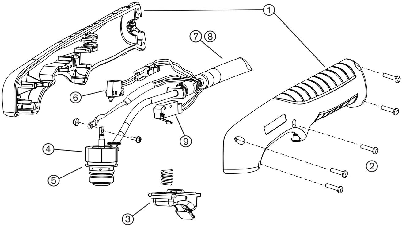
The entire hand torch and lead assembly can be replaced, or individual component parts can be replaced. Part numbers starting with 088 indicate complete torch and lead assemblies.
