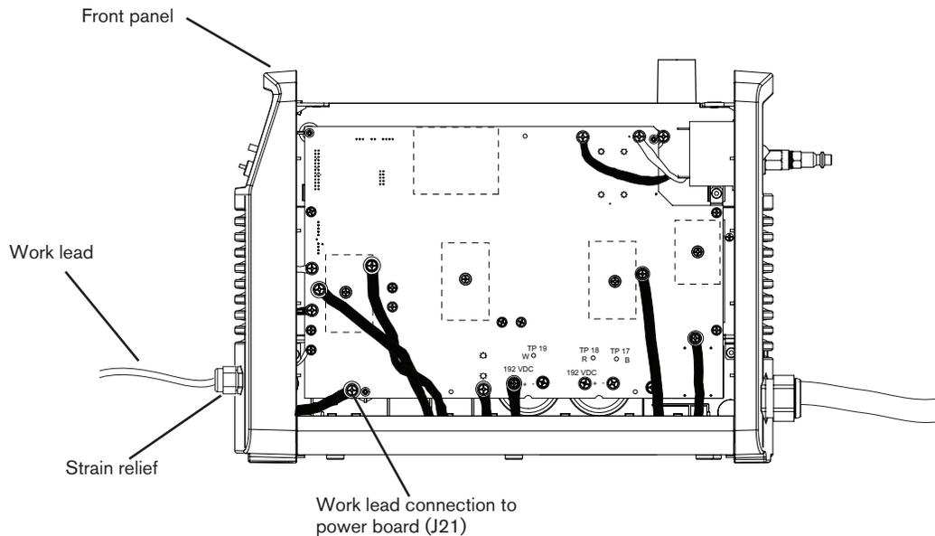
5. Thread the connector end of the new work lead through the front panel and fit the strain relief into the hole in the panel.
