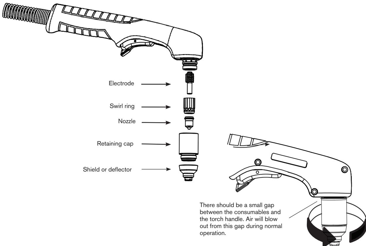
Note: Tighten only to finger-tight. Overtightening will cause the torch to misfire.
