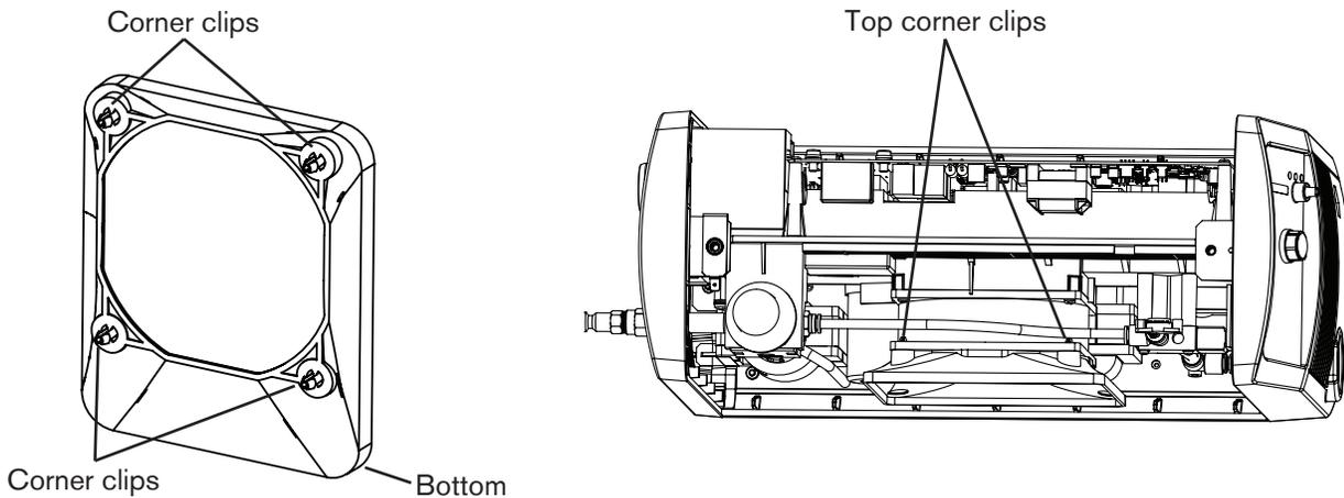
6. Slide the old fan out from the power supply.
