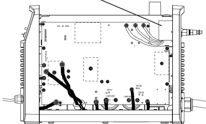
5. Remove the screw that holds the green/yellow ground wire to the heatsink.
