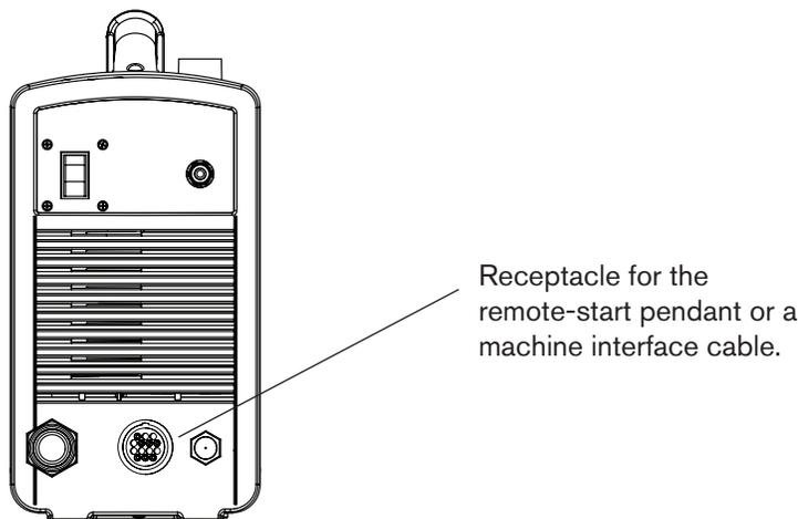
Receptacle for the remote-start pendant or a machine interface cable.
