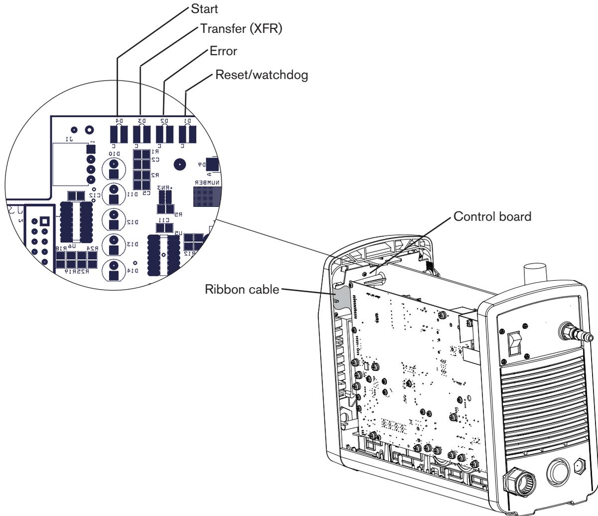
The control board LEDs are:
