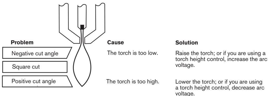
Notes: The squarest cut angle will be on the right side with respect to the forward motion of the torch. The left side will always have some degree of bevel.
