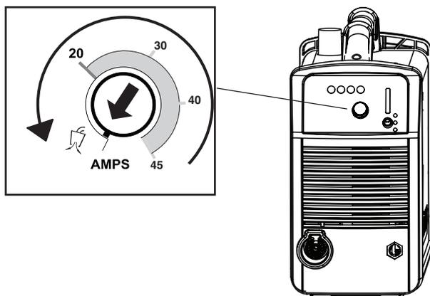
2. With the amperage knob in the gas test position, pull up on the pressure regulator knob on top of the system to unlock it.
