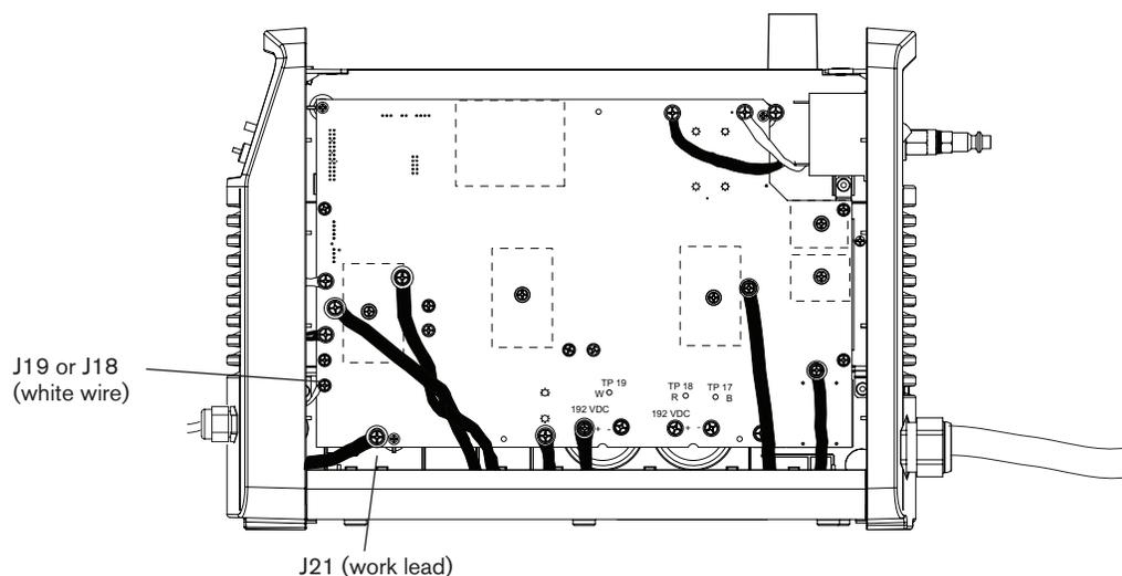
14. Replace the Mylar barrier in front of the power board. Replace the rear panel and secure it with the screw. Replace the cover.
