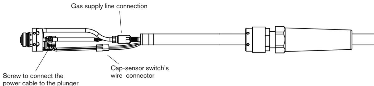
4. Use a #2 Phillips screwdriver and a 1/4-inch nut driver (or adjustable wrench) to remove the screw and nut that secure the torch's power cable to the plunger. (Turn the plunger if necessary to gain access to the screw.)
