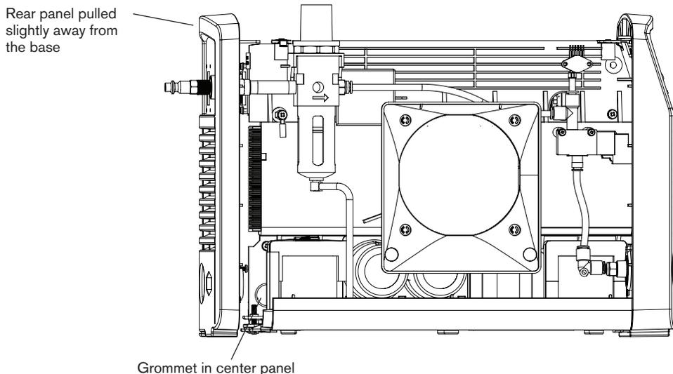
10. Route the wires along the base of the unit and behind the cables connected to the power board.
