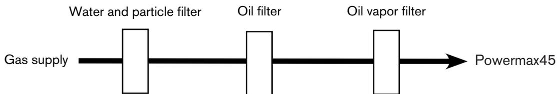
The filtering system should be installed between the quick-disconnect coupler and the power supply.
