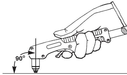
2. Press the torch trigger to start the arc. Pause at the edge until the arc has cut completely through the workpiece.
