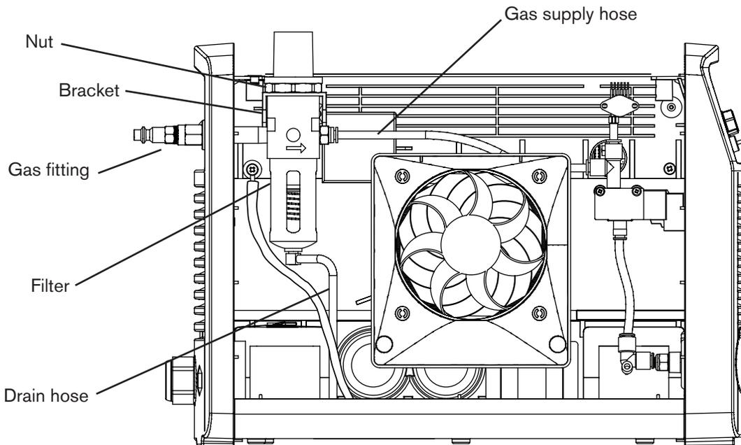
6. Unscrew the nut that holds the air filter in the bracket. Tip the bottom of the air filter away from the power supply and slide the filter out of the bracket.
