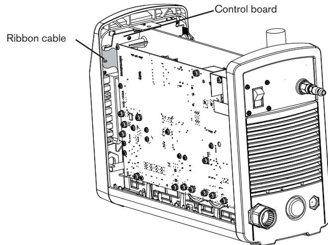
9. Screw the new control board into place with the 3 retaining screws and then attach the ribbon cable.
