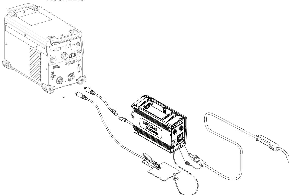
**CrossLinc™** - CrossLinc is a new welding system communication technology. When using a CrossLinc enabled power source such as the FX360XL and a CrossLinc enabled wire feeder such as the LN-25X, welding voltage can be controlled remotely without the use of an additional control cable.
