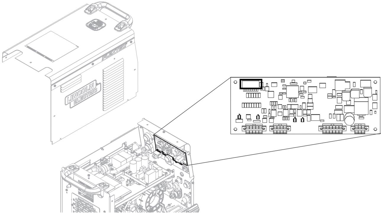
The User Interface pc board has one bank of dip switches. As shipped from the factory and under normal conditions, the dip switches are all in the 'off' position. There are 3 instances that require a change of the dip switch.
