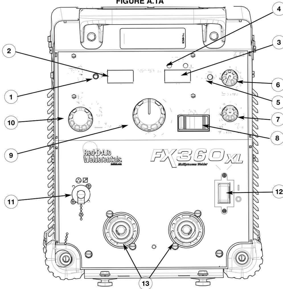
1. **Thermal LED:** A yellow light that comes on when an over temperature situation occurs. Output is disabled until the machine cools down. When cool, the light goes out and output is enabled.
