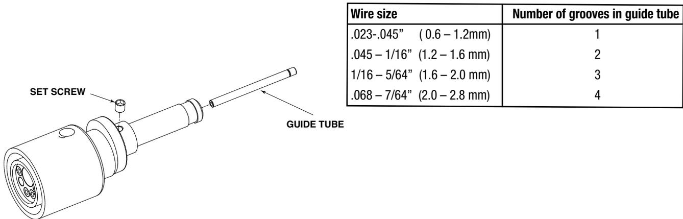
9. Slide the Oxo or FastMate gun adapter into the wire drive and secure with the thumb screw.
