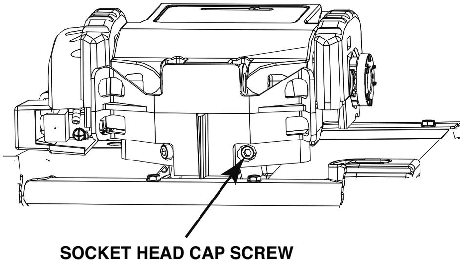
3. Rotate the wire drive to the desired position and tighten the screw.
