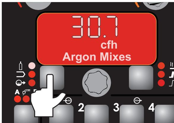
To display the actual gas flow, press the left button to select the shielding gas LED and then press the gas purge button. To display gas flow while welding, change P.3 in the set-up menu to "Show Gas Flow Rate."
