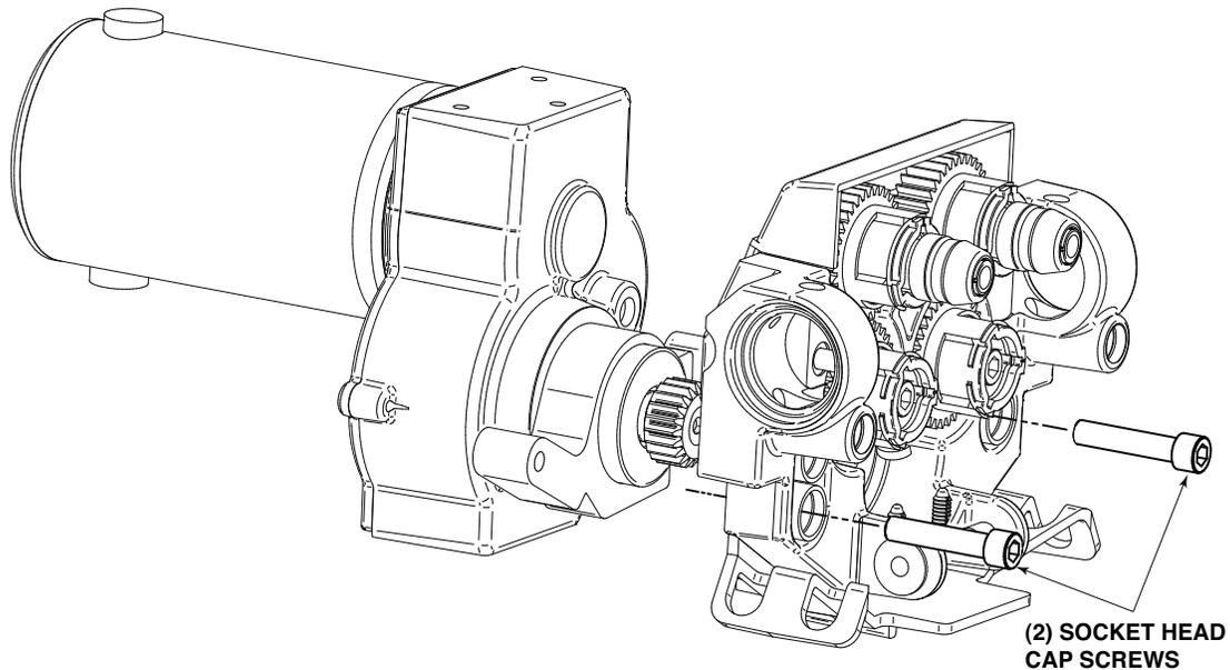
4. Remove the screw holding the pinion gear using a Phillips screw driver. Remove the pinion gear.
