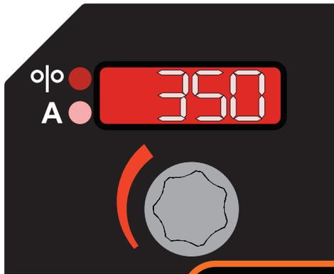
The left display and knob are used to adjust either wire feed speed or amperage, depending upon the process selected.
