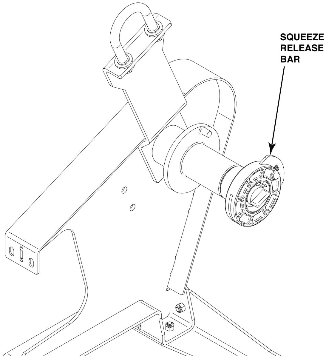
3. Place the spool on the spindle, aligning the spindle brake pin with one of the holes in the back side of the spool. An indicator mark on the end of the spindle shows the orientation of the brake holding pin. Be certain the wire feeds off of the spool in the proper direction.
