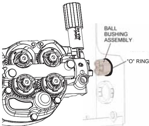
3. Remove the three socket head cap screws from the ball bushing assembly. **Caution: as the screws are being loosened, the balls may fall free from the assembly.** Remove the balls and the steel washer.
