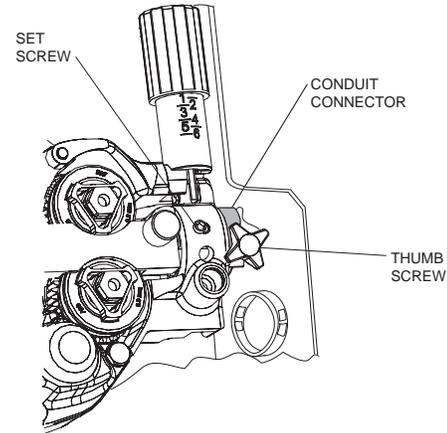
5. Insert the conduit connector into the feed plate and secure with the set screw. Rotate the conduit connector so the thumb screw does not interfere with the idle arm or door.
