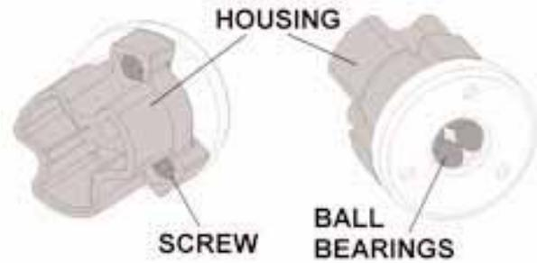
4. Place the ball bushing housing into the wire feeder case and secure with the "O" ring.
