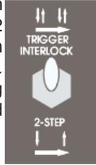
Place the toggle switch in the DOWN position for 2 Step operation or in the UP position for Trigger Interlock operation.
