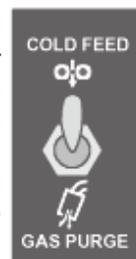
Hold the toggle switch in the DOWN position to activate Gas Purge and let the shielding gas flow. The gas solenoid valve will energize but neither the power source output nor the drive motor will be turned on. The Gas Purge switch is useful for setting the proper flow rate of shielding gas. Flow meters should always be adjusted while the shielding gas is flowing.
