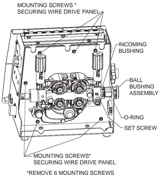
2. Remove the o-ring holding the ball bushing assembly to the back of the wire feeder. Remove the ball bushing assembly.
