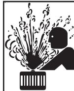
1.h. To avoid scalding, do not remove the radiator pressure cap when the engine is hot.
