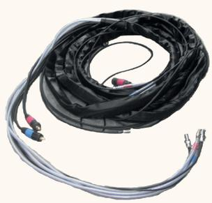
To increase the operating distance between the welding head and the SAXX power source, we offer cable extensions. In order to guarantee the proper functioning of the machine, a **maximum length of 20m of extension or a maximum quantity of 2 extension cables** is recommended. For a higher need, please consult us.
