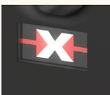
When the power source is powered on and the head connected, the light is on steady. When the machine is welding, the indicator light flashes.
