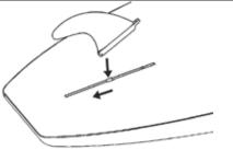
STEP 5 – ROTATE THE FRONT EDGE OF THE FIN DOWNWARDS AND ALIGN THE METAL TAB WITH THE HOLE IN THE FRONT OF THE FIN. ONCE ALIGNED, INSERT THE PHILLIPS SCREW IN THE HOLE AND TIGHTEN. AS A GENERAL RULE, IF YOU WANT YOUR BOARD TURN MORE EASILY, MOVE THE FIN FORWARD. IF YOU WANT IT TO TRACK BETTER, MOVE IT REARWARD. OBRIEN RECOMMENDS STARTING AT NEAR CENTER AND ADJUSTING AS NEEDED.
