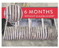
ScaleBlocker® is recommended for steamers to help minimize limescale buildup and corrosion, which can significantly impact the operation of your equipment, resulting in downtime or service calls. It's a safe and economical way to maintain your investment.
