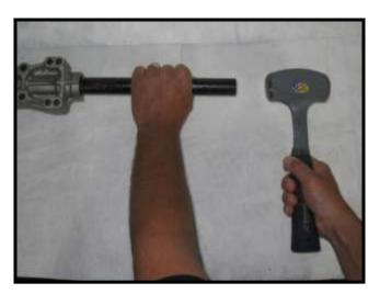
4. Correct position of axle bushing = 2~3mm beyond offset in upper housing.
