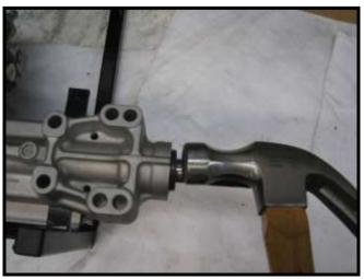
10. Use a box end wrench with outer diameter near same size as seal to drive the seal to its final resting position.
