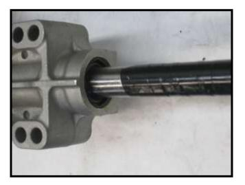
12. Remove tape after seal has been pressed to final position.
