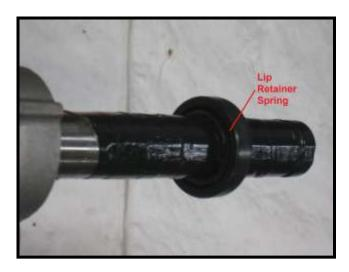
8. Use a box end wrench and hammer to move seal to final position.
