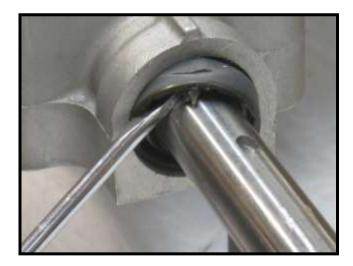
2. An out of position axle bushing can cause seal lip deformation and/or damage; thus, resulting in oil leakage.
