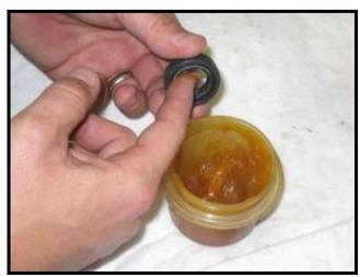
7. Slide seal onto wrapped axle shaft. Seal side with lip retainer spring should be on inboard side.
