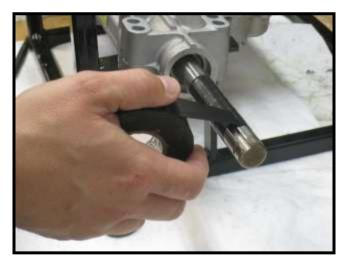
6. Apply a generous coating of grease between the double lips of new seal and over the newly applied tape on axle.
