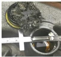
If present, inspect differential side gears for heavy wear or missing portions of the teeth.
