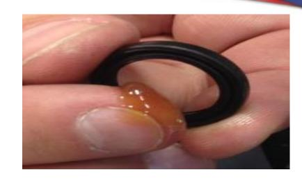
Install the Seal by hand and push in firmly. Make sure the flat side of the Seal is facing the outside of the Housing
