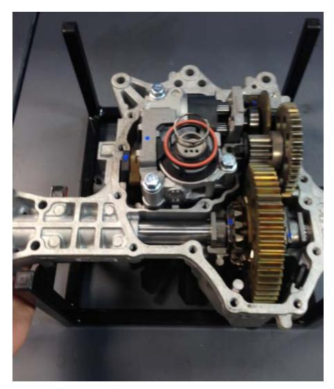
The charge pump should be in the "FROWN" position in order to be in the correct orientation.
