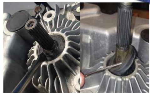
Remove the Snap Ring. **Note:** The internal Snap Ring can almost always be retained and reused
