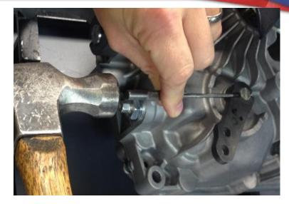
Remove the Bypass Arm and Roll Pin. Wipe the area clean of debris before installing the new Arm
